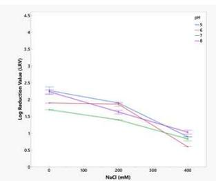
Figure 3: Effect of pH and NaCl concentration on LRV for the plate-based screening.
