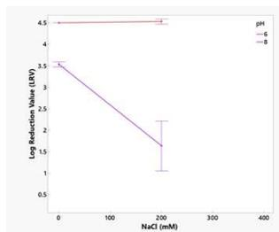
Figure 4: Effect of pH and NaCl concentration on LRV for the bench screening.
