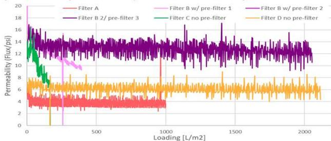
Filters A and D had little flow decay with no specialized pre-filters. Filter B had two pre-filter options where there was little flow decay. Filter C was only tested without a pre-filter due to long lead times of the pre-filter. Throughput may be improved with the addition of a pre-filter.
